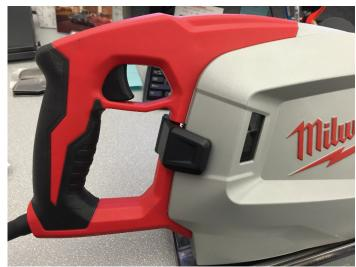
**Serial 'D' Construction-**If the tool you are servicing looks like this, use Bulletin No. 54-40-1628
